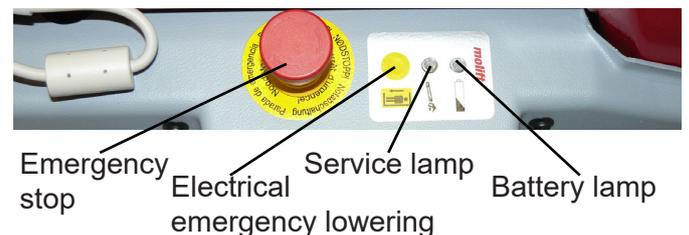
On the right side of the chassis there is a service light which will give a signal when the lifter needs service. When there is a green light, the lifter can be used normally. If there is no light, push one of the up/down buttons to activate the electronics, and the service lamp will illuminate. See the chapter "Maintenance".
