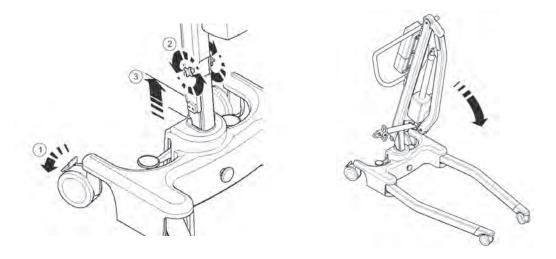
4. Lift the folded Advance upright (using the legs and push handle as a guide) being careful that the mast and boom stay together as you tilt upright.
