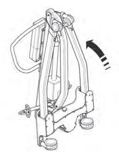
5. Pull the restraining strap sharply upwards and extend over the wheels. (This will keep the legs, mast and boom neatly together during transit and storage).
