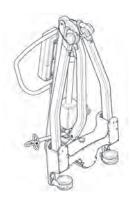
2. Release the leg and mast assembly by unfastening the restraining strap from the wheels. This strap will retract neatly into the top of the mast section.
