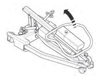
4. Lift the mast assembly upright (using the top of the push handle), and drop the mast into the slot, aligning the mast engagement decals (1), tighten mast lock knobs (2), release braked castors (3).
