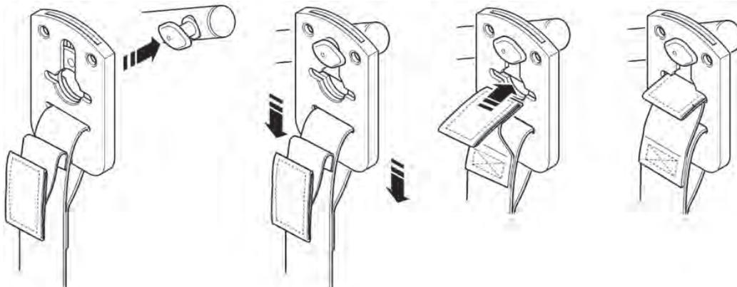
Securi3 sling attachment system. Example of installation.
