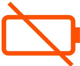
The empty battery symbol showing on the display indicates that the battery has no capacity left and should be placed on charge immediately.
