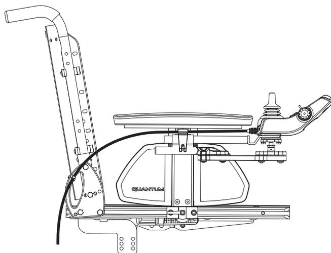
Figure 9. Controller Harness Routing on a TB-Flex Seat
